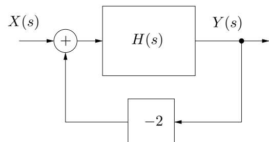
$$G(s) = \frac{as + 5}{s^2 + 3as + 10a + 2(as + 5)}, \quad \frac{\partial G}{\partial a} \frac{a}{G} = \left. \frac{a(s^3 - 15s - 50)}{(as + 5)(s^2 + 5as + 10 + 10a)} \right|_{s=0, a=0.5} = -1/3$$
