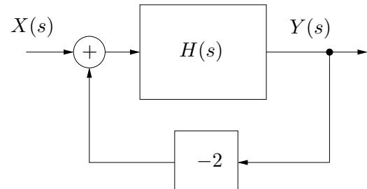
$$G(s) = \frac{2as + 10}{s^2 + 6as + 5a + 2(2as + 10)}, \quad \left. \frac{\partial G}{\partial a} \frac{a}{G} \right|_{s=0, a=0.2} = \left. \frac{a(s^3 - 30s - 25)}{(as + 5)(s^2 + 10as + 20 + 5a)} \right|_{s=0, a=0.2} = \frac{-1}{21}$$
