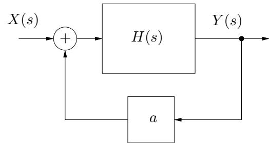
$$G(s) = \frac{2s + a}{s^2 - 6as - 3a - a^2}, \quad \frac{\partial G}{\partial a} \Big|_G = \frac{a(13s^2 + 6s + 4as + a^2)}{(2s + a)(s^2 - 6as - 3a - a^2)} \Big|_{s=0} = \frac{-a}{a+3} \Big|_{a=1} = -1/4$$
